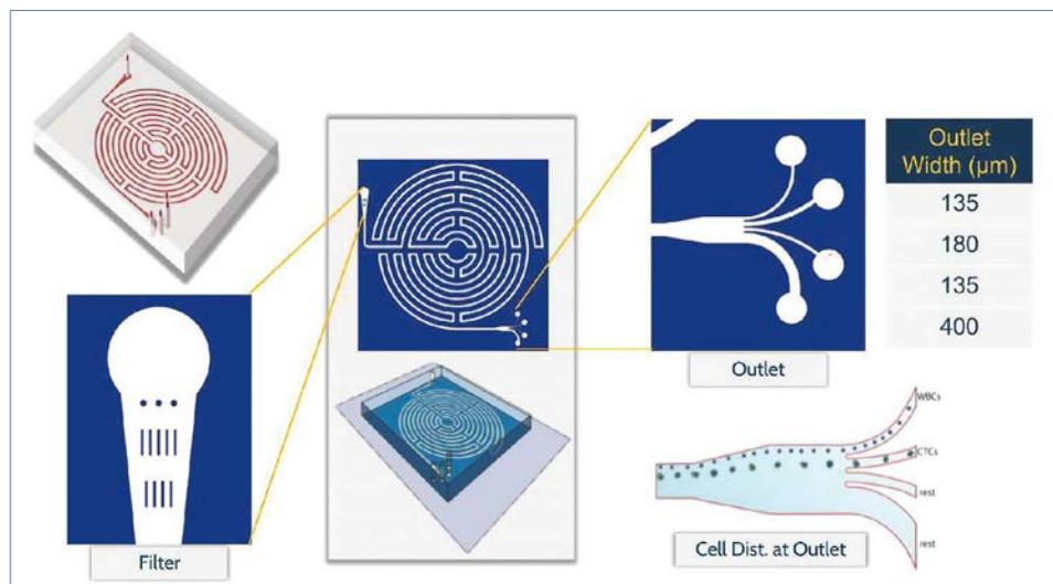
A microfluidic device for the separation of CTCs has been developed by Sunitha Nagrath, Ph.D., and colleagues at the University of Michigan. The device, which is depicted in this schematic, incorporates a labyrinthine path that subjects small cells (such as healthy blood cells) and large cells (such as CTCs) to different forces, channeling the cells to different streamlines.
