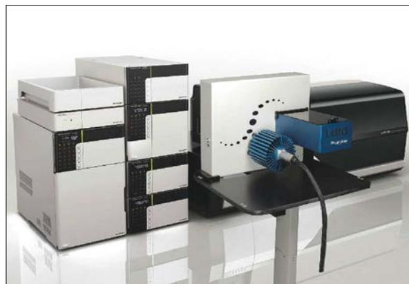
This new high-speed platform will significantly improve productivity in high-throughput laboratories performing toxicology, drug discovery, and food safety applications. It incorporates the LDTD (laser diode thermal desorption) ion source technology and is designed to synchronize with the speed of the Shimadzu LCMS-8060 triple quadrupole mass spectrometer. The platform ionization mode selector allows users to rapidly switch
