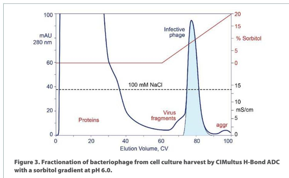
**Figure 3. Fractionation of bacteriophage from cell culture harvest by CIMultus H-Bond ADC with a sorbitol gradient at pH 6.0.**
