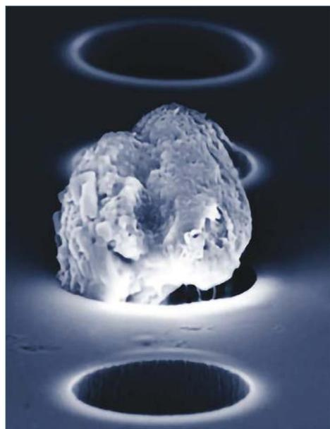
At the University of Miami, researchers in the laboratory of Richard J. Cote, M.D., are developing next-generation filter technology for the capture of viable circulating tumor cells (CTCs). By introducing novel pore architectures such as “slot” pores and double-membrane microfilters, the researchers can avoid procedures that complicate functional characterization, such as fixation in 1% formalin.
