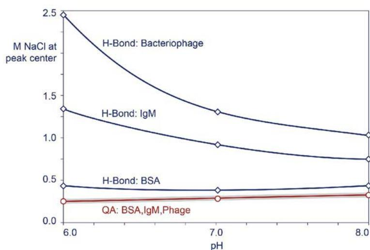
Figure 1. Elution of proteins and virus particles from CIMultus™ H-Bond™ ADC and CIMultus QA as a function of pH.
